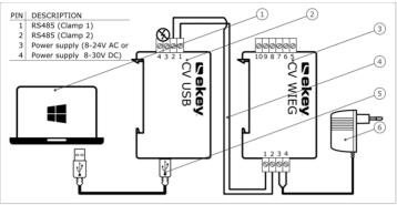
Fig. 6: Wiring diagram for configuring the converter
