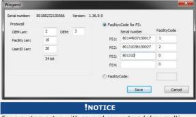
For a system setup with several converters (*ekey multi* variant 2), input field **FS1** must always be used for the finger scanner assignment.
